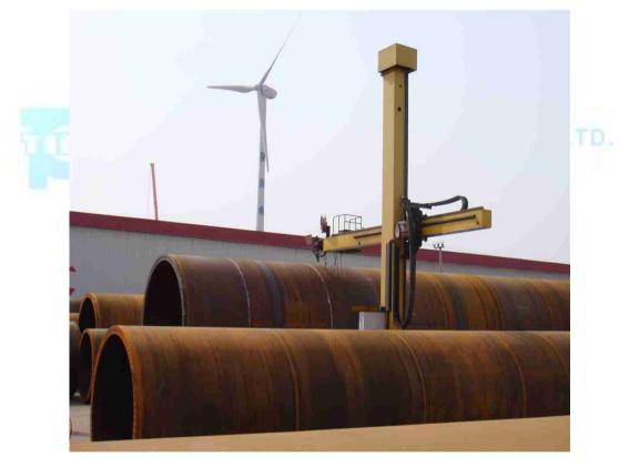
Welding manipulator used in wind power industry
