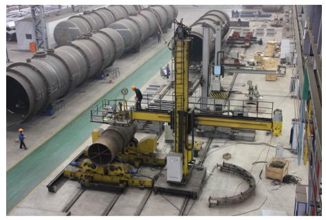
Welding manipulator used in pressure vessel industry
