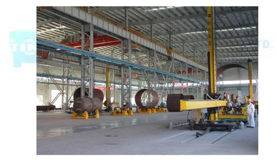
Welding manipulator used in petroleum industry
